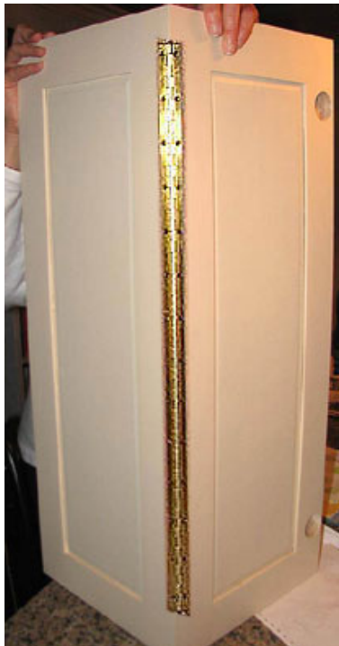
Figure 1: Piano Hinge Configuration
